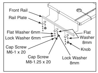
Figure 3. Installing front rail onto table.
